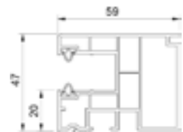
One-sided (PVC) roller guide - RS revision from the inside.
