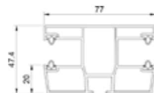
Divisive (PVC) roller guide - RS revision from the inside.
